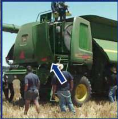
Baydur® 730S IBS rear door (12 kg) of John Deere Combine Al-mold with Ni-shell
