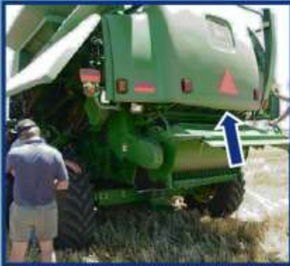
Baydur® 730 IBS rear flap (30 kg) of John Deere Combine Al-mold with Ni-shell
