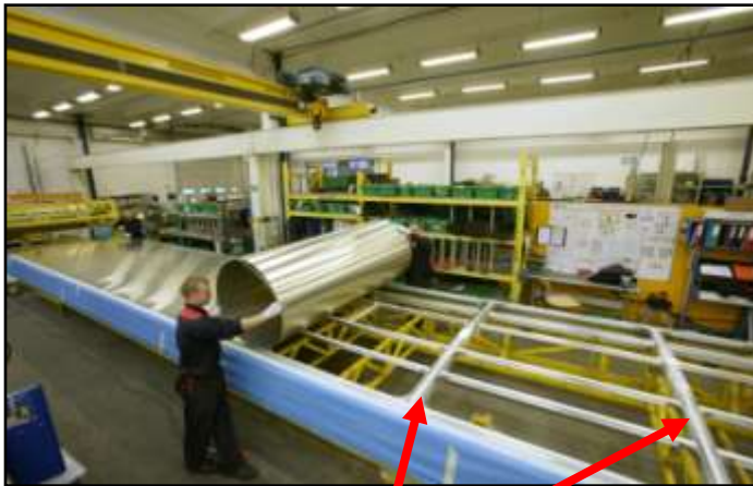
One piece aluminium roof bonding
